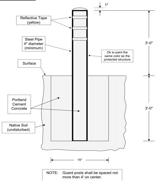
Guard post to be completely filled with concrete. 2016 CFC 312
