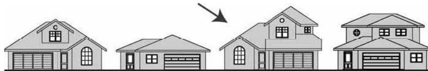
The revised design became compatible with its neighbors by stepping back the second story and providing variation in the roof and building forms.
