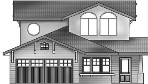
These new second-story windows are of different shape and proportions and material (metal vs. original wood) than the original first-story and do not appear compatible.
