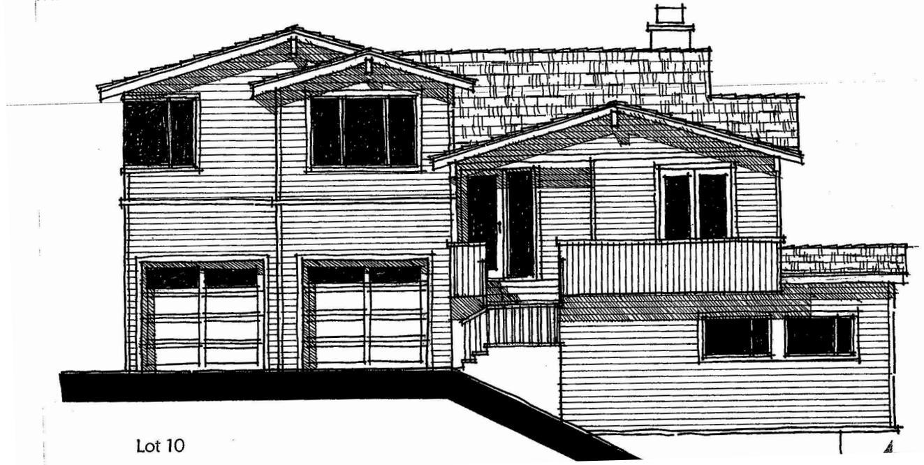
Note: The approved front elevation shows the 2 garage doors of the proposed 2-car garage with 1-tandem space.
