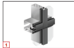
1 CURTAIN WALL KAWNEER CLEARWALL 2-1/2"X8" DARK GREY MATTE EXTRUDED AL MULLIONS DOUBLE-PANE CLEAR LOW-E SOLARBAN 70XL GLAZING
