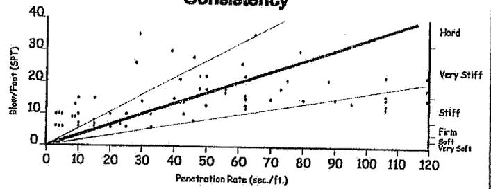
\* Seconds per foot, based on a portable percussion rig advancing a 1 1/2-inch diameter split-spoon sampler with a force of 35 ft. lb. at a rate of 1270 blows per minute.
