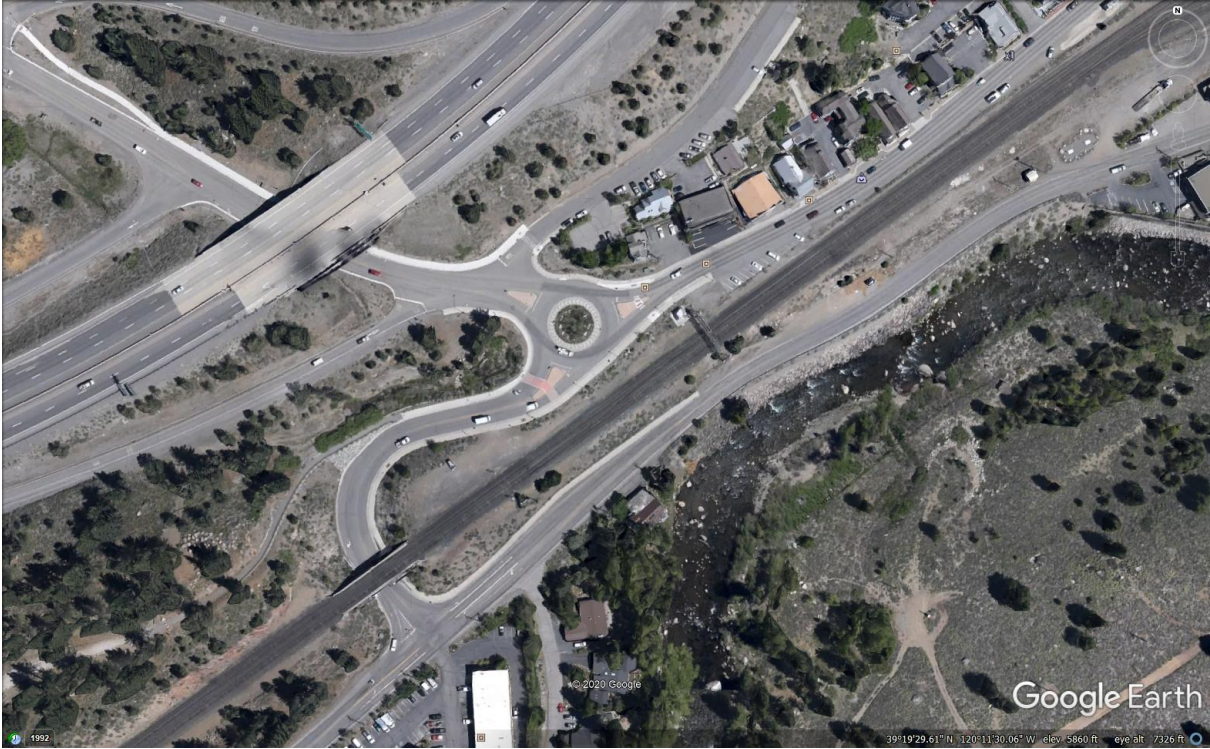
Example of traffic calming on high speed roundabout approach (SR 89 north/ Prosser Dam Rd/ Alder Drive - example from Dan Wilkins)
