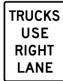
Figure 8: Trucks Use Right Lane Signage (R4-5)
