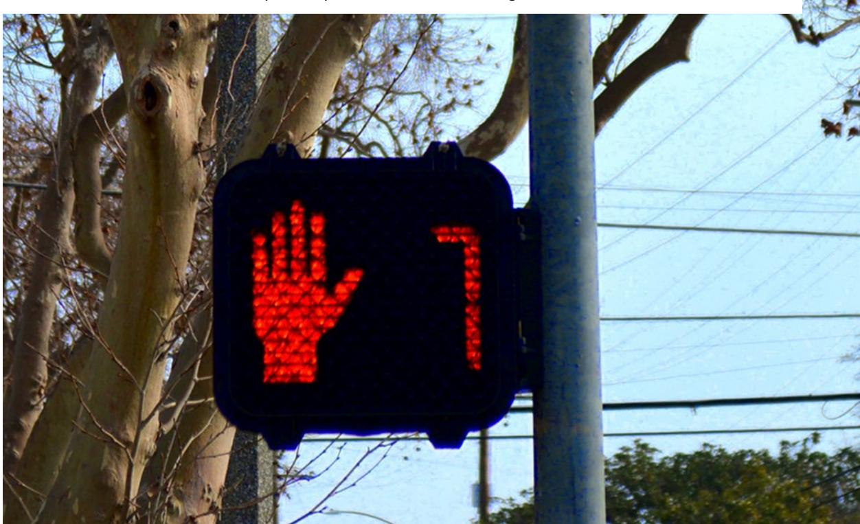
Example of a pedestrian countdown signal head
