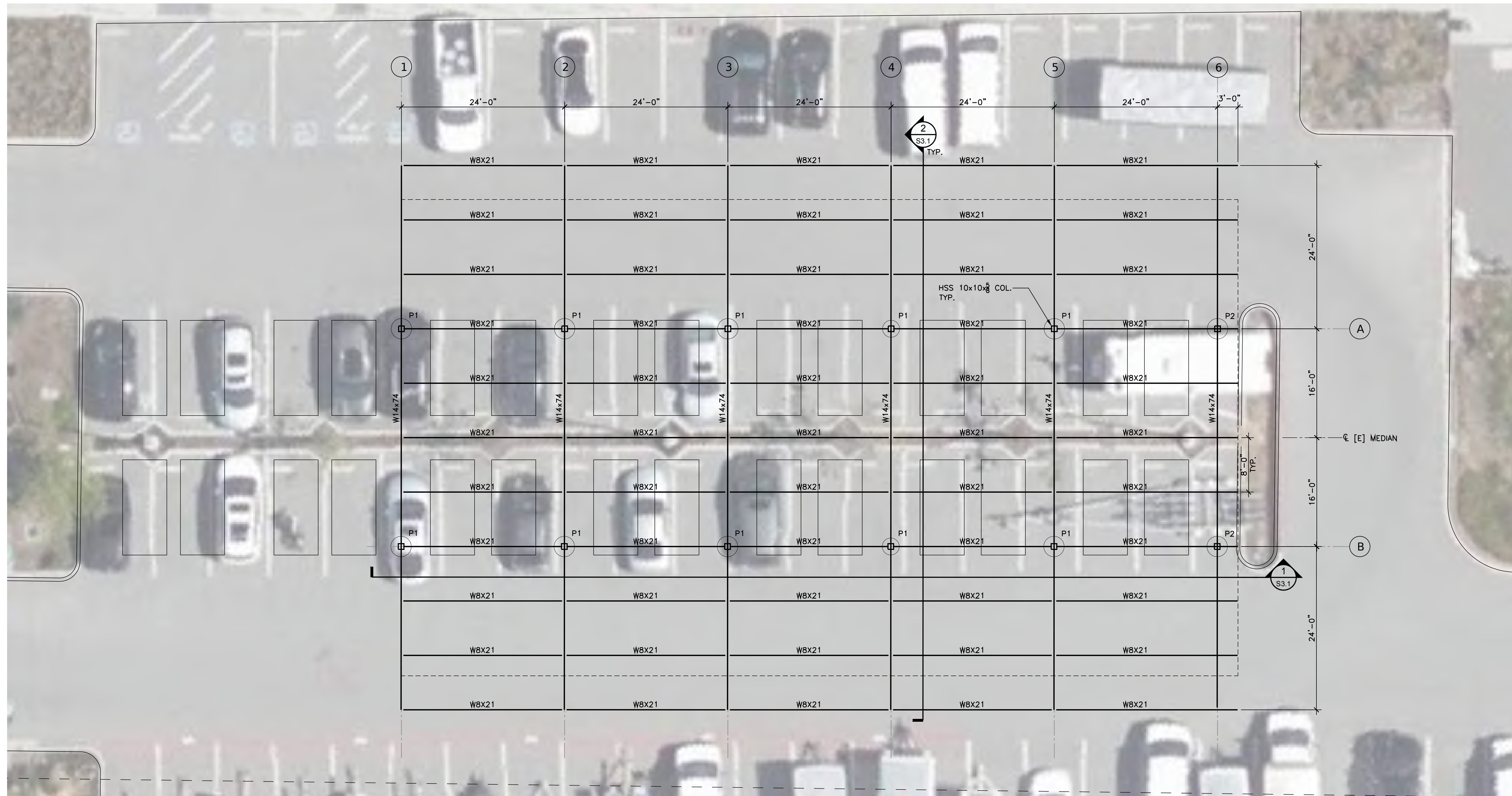
1 SOLAR STRUCTURE FRAMING PLAN 1/8"=1'-0"
