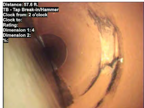
10, 00:04:01, 57.60ft Tap Break-in/Hammer at 2 o'clock, dia/height: 4.000inch, within 8 inch
