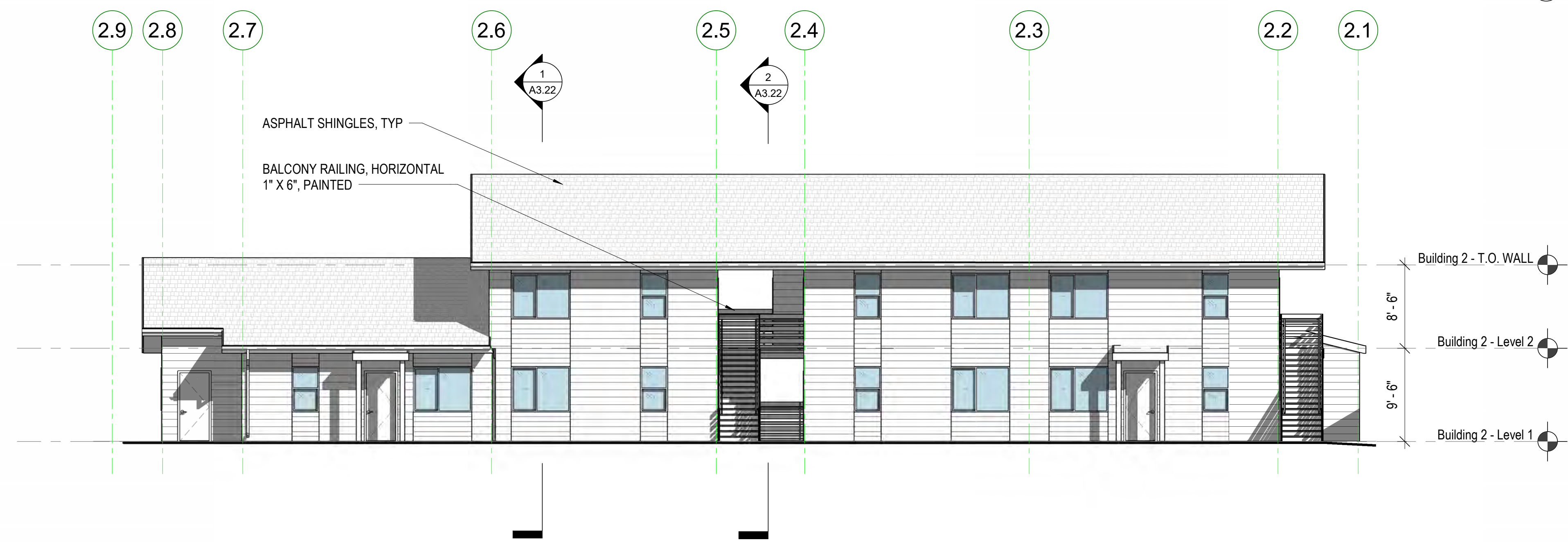
BUILDING 2 - EAST ELEVATION 1/8" = 1'-0"
