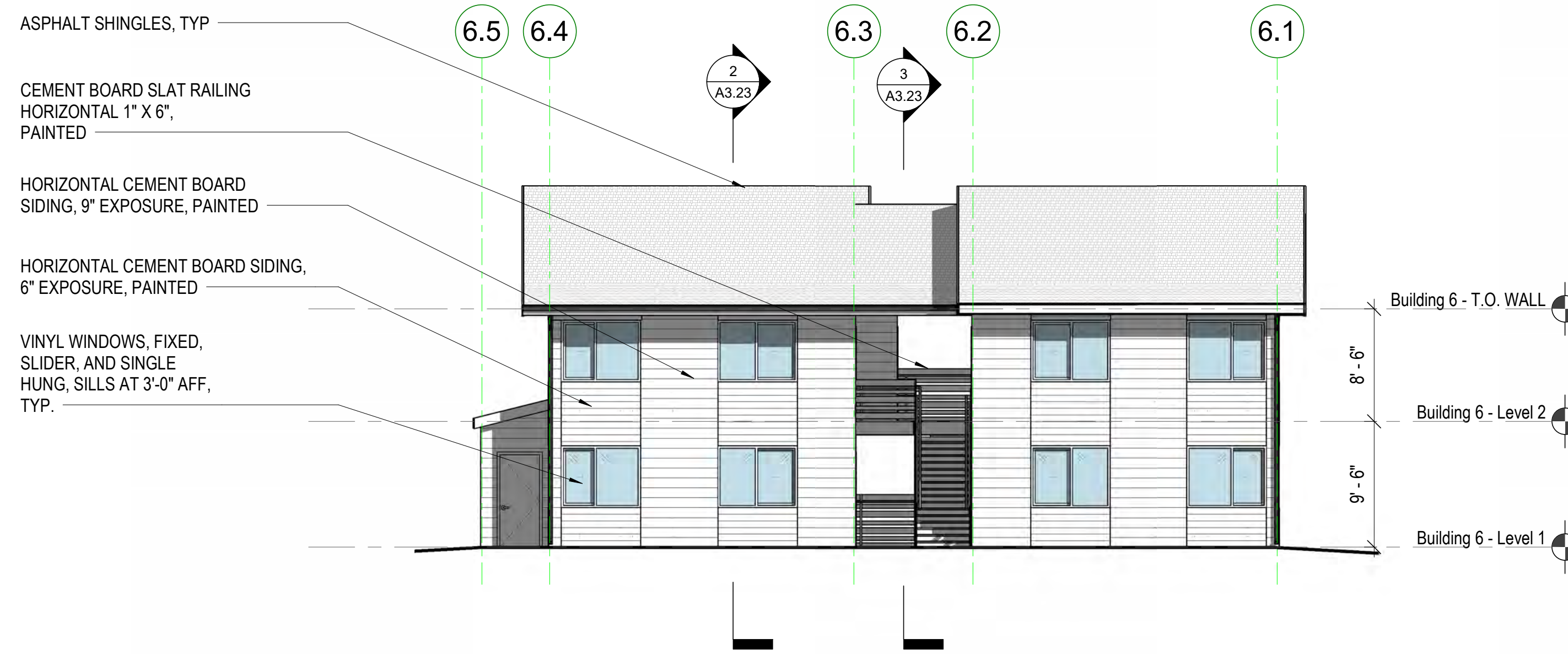
BUILDING 6 - NORTH ELEVATION 1/8" = 1'-0" ④
