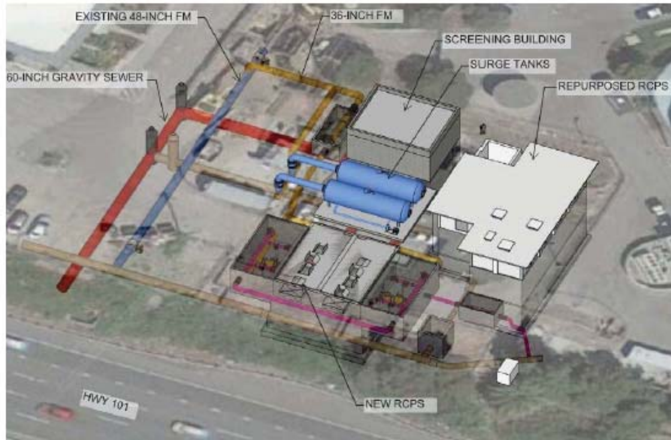
Figure ES-2. Overall RCPS layout – plan view
