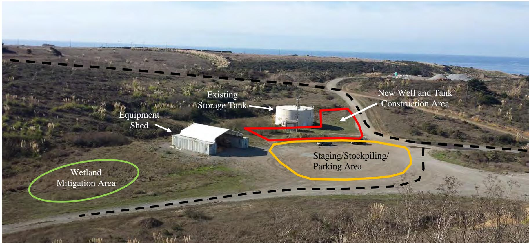
**Photo 1** – Photo of project area looking northwest, showing proposed new storage tank and well location, staging and material storage area, and proposed wetland mitigation site. Access road locations are indicated by dashed lines. The Quarry Pond is immediately to the left of the photo.
